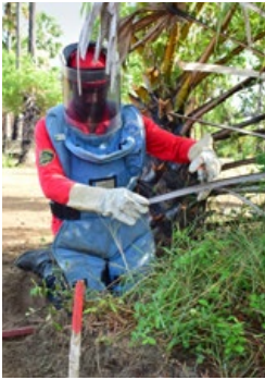
Thick vegetation and numerous metal parts in the ground hinder mine detection.
