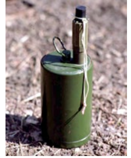
Bounding mine, type 69: When detonated, a propelling charge launches the body of the mine about a metre into the air, where the main charge then explodes, spraying shrapnel all around.
